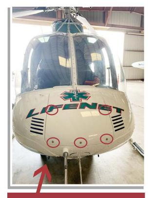
Use a screwdriver to open the five fasteners on the front of the battery compartment.
