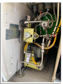
The oxygen system contains 3000 liters of gaseous oxygen.
