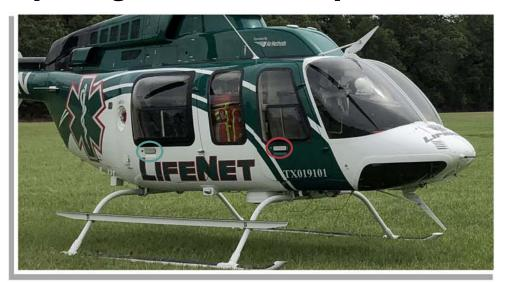
There are two door handles on the pilot side of the aircraft.
